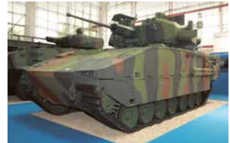
A further enhanced IFV has lately been presented. Sharing the outstanding ergonomics and passive protection, this ASCOD version features an unmanned turret, EuroTrophy APS, EuroSpike ATGM launcher, MESHnet® V6 Tactical CIS, and optional composite rubber tracks.
