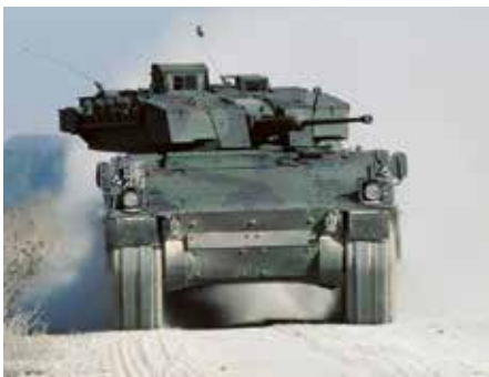
The basic IFV version holds an infantry squad of up to eight and can be armed with a wide variety of manned or unmanned turrets for autocannons up to 30/40 mm. Austria's fleet is currently undergoing a comprehensive life cycle extension program.
