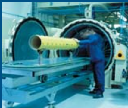
Processing motor case insulation on ESSM
