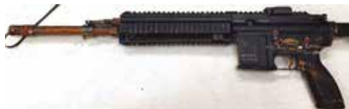
HK416 protected with oil only during Salt Fog Test
